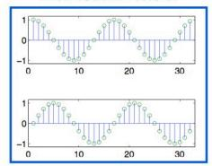
A *shifted* sinusoidal vector can be written as a weighted sum of two *fixed* sinusoidal vectors!
