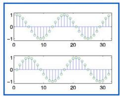
A *shifted* sinusoidal vector can be written as a weighted sum of two *fixed* sinusoidal vectors!
