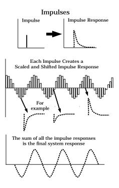
Figure 2: Characterizing a linear system using its impulse response.
