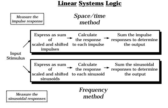
Figure 6: Alternative methods of characterizing a linear system.
