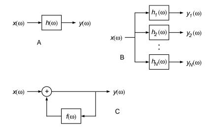
**Figure 8:** Block diagrams of linear filters. A: Linear filter with frequency response  $\hat{h}(\omega)$ . B: Bank of linear filters with different frequency responses. C: Feedback linear system.
