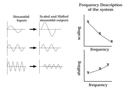
Figure 5: Characterizing a system using its frequency response.
