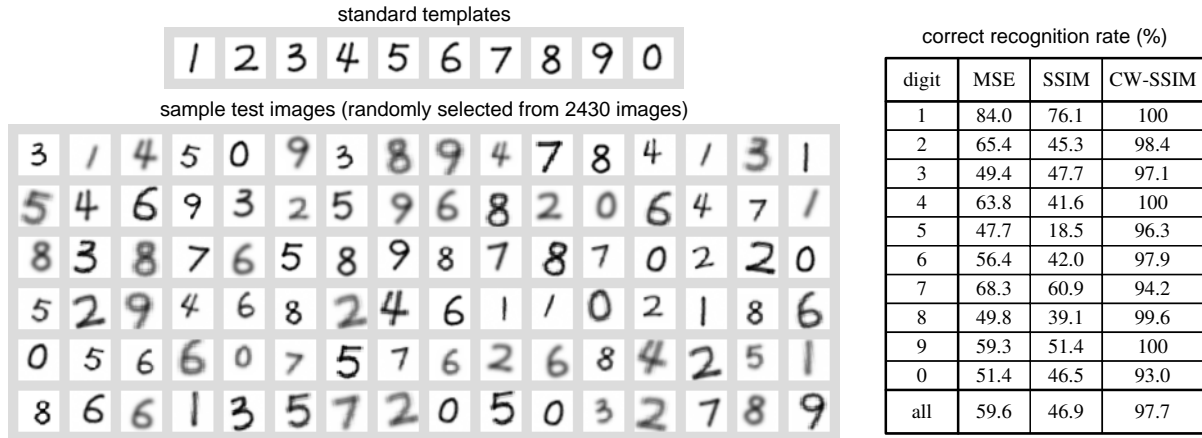
Fig. 2. Pattern matching without registration. Each test image (from a database of 2430 images) is matched to the ten standard templates using MSE, SSIM and CW-SSIM as the similarity measures, without any normalization or registration process in the front. The test image is then “recognized” as belonging to the category that corresponds to the best similarity score. The resulting correct recognition rates show that both MSE and SSIM are sensitive to translation, scaling and rotation of images, but CW-SSIM exhibits much stronger robustness.
