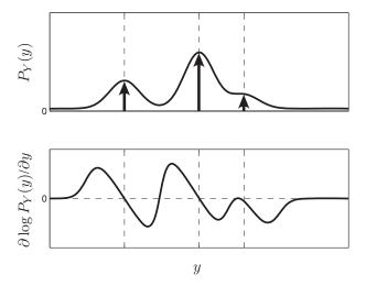
Figure 1: Illustration of the NEBLS estimator for a one-dimensional value with additive gaussian noise. (Top) Measurement density,  $P_Y(y)$ , arising from a signal with prior consisting of three point masses (indicated by upward arrows) corrupted by additive gaussian noise. (Bottom) Derivative of the log measurement density, which, when added to the measurement, gives the NEBLS estimator (see equation 2.4).
