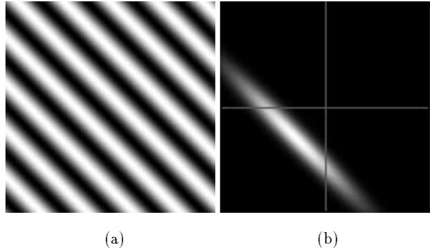
**Figure 2:** (a) One frame of a drifting sin grating sequence. The normal direction of the motion was down and to the left. The drift speed (in the normal direction) was 0.83 pixel/frame. (b) The response of the system computed over a patch near the center of the image. The peak of the response coincides with the actual normal velocity.
