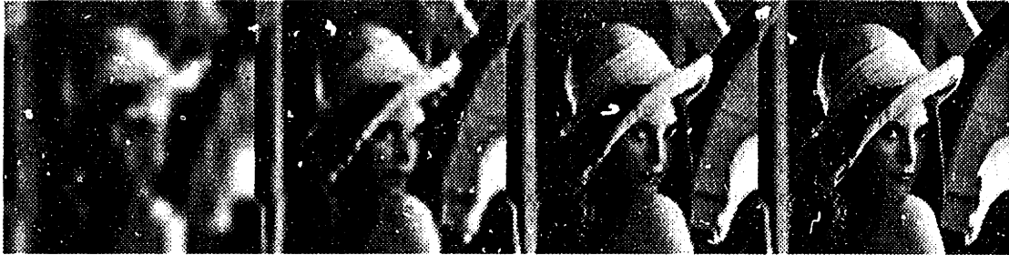
Figure 22: Progressive transmission images for a four-level pyramid transform using 9-tap separable filters. The first image is produced by reconstructing only the lowpass signal at the fourth pyramid level. The next image results from reconstructing the entire fourth level, or equivalently, the lowpass image on the third level. Bit rates (entropies) are: 0.03, 0.09, 0.24, and 0.49 bits/pixel and the image size is 256 \times 256 . The final image at 0.65 bits/pixel is not shown.
