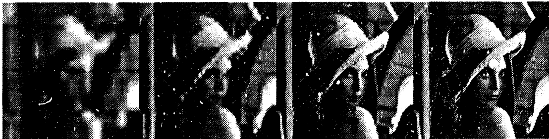
Figure 23: Progressive transmission images for a four-level pyramid transform using 15-tap separable analysis filters and 3-tap separable synthesis filters. Bit rates are essentially the same as for the 9-tap example above.
