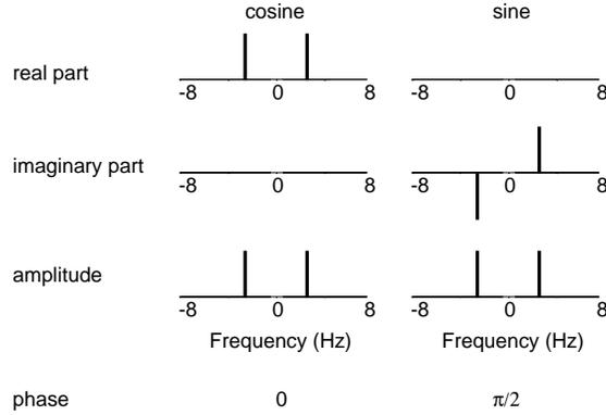
**Figure 10:** Fourier transforms of sine and cosine signals. The amplitudes are the same, but the phases are different.
