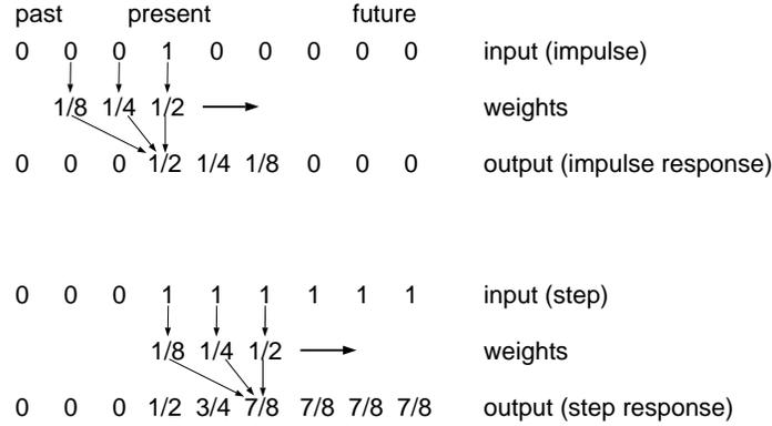
**Figure 3:** Convolution as a series of weighted sums.
