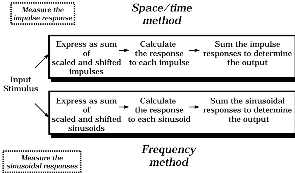
**Figure 6:** Alternative methods of characterizing a linear system.
