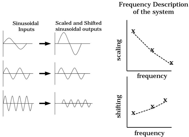
**Figure 5:** Characterizing a system using its frequency response.
