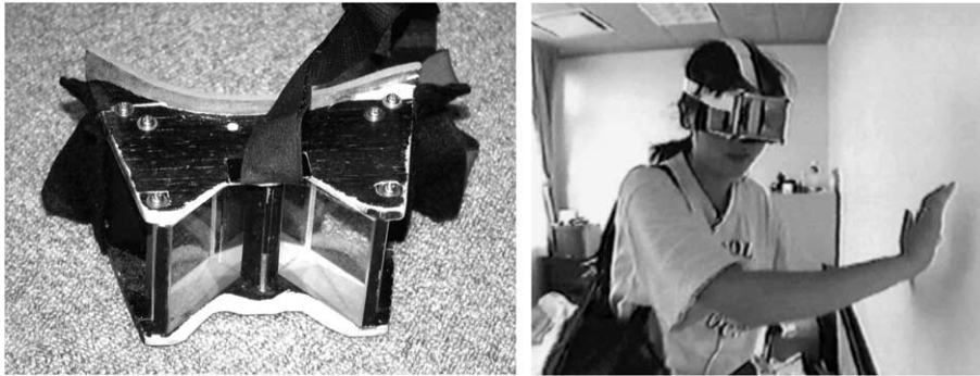
Fig. 2. Left–right reversing goggles (left) and one of the four subjects who wore the goggles (right). They wore the goggles for more than five weeks, except while they slept.
