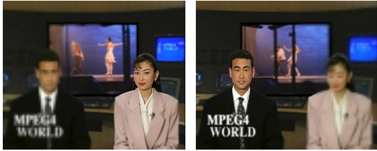
Simulations of the high spatial resolution in central vision coupled with the blurry low spatial resolution in the periphery.
