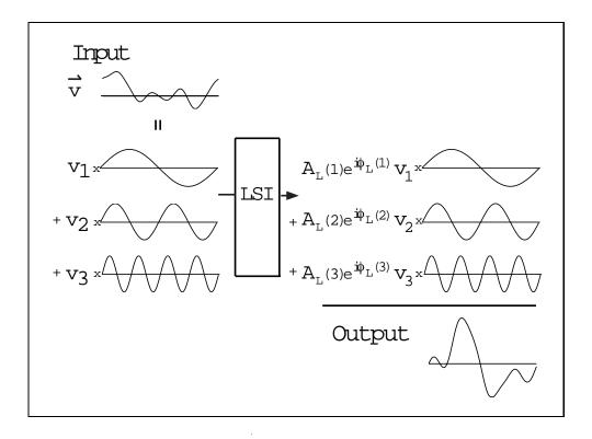
the amplitude by a factor  $A_r(k)$  and shift the phase by an amount  $\phi_r(k)$ . Finally, the system response is a sum of sinusoids with amplitudes/phases corresponding to
