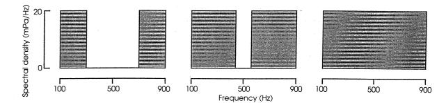
The noise on the left has a wide notch, whereas the middle one has a narrow one. These are known as *notched noise*. The noise on the right has no notch at all; it has a constant spectral density over the frequency range of interest.
