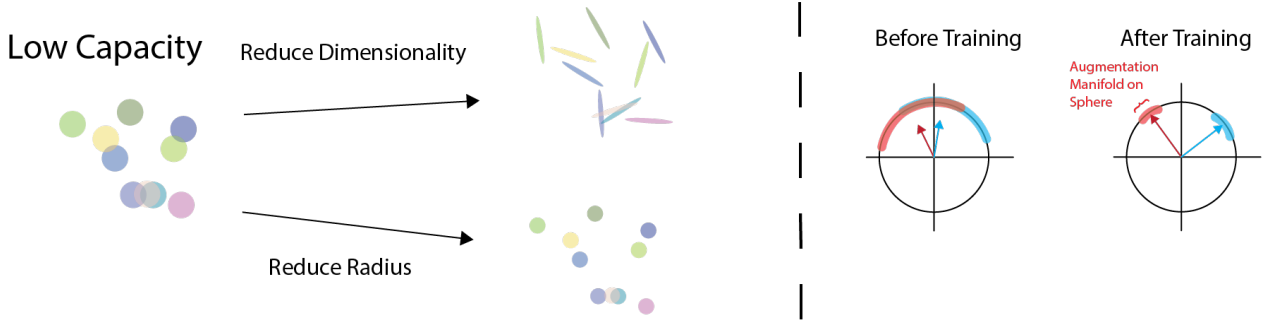
Figure 1. Two dimensional illustrations of high and low capacity representations. Left: the capacity (linear separability) of a random set of elliptical regions can be improved, either by reducing their sizes (while maintaining their dimensionalities), or by reducing their dimensionalities (while maintaining their sizes). Right: the objective proposed in this paper aims to minimize the nuclear norm (product of size and sqrt dimensionality) of normalized data vectors (ie., lying on the unit sphere). Before training the manifolds have a large extent and thus the matrix of their corresponding centroid vectors has low nuclear norm. After training the capacity is increased. The manifolds are compressed and repelled from each other, resulting in centroid matrix with larger nuclear norm and lower similarity.
