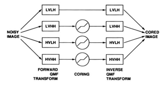
Figure 4-2: Information flow in coring (one level).
