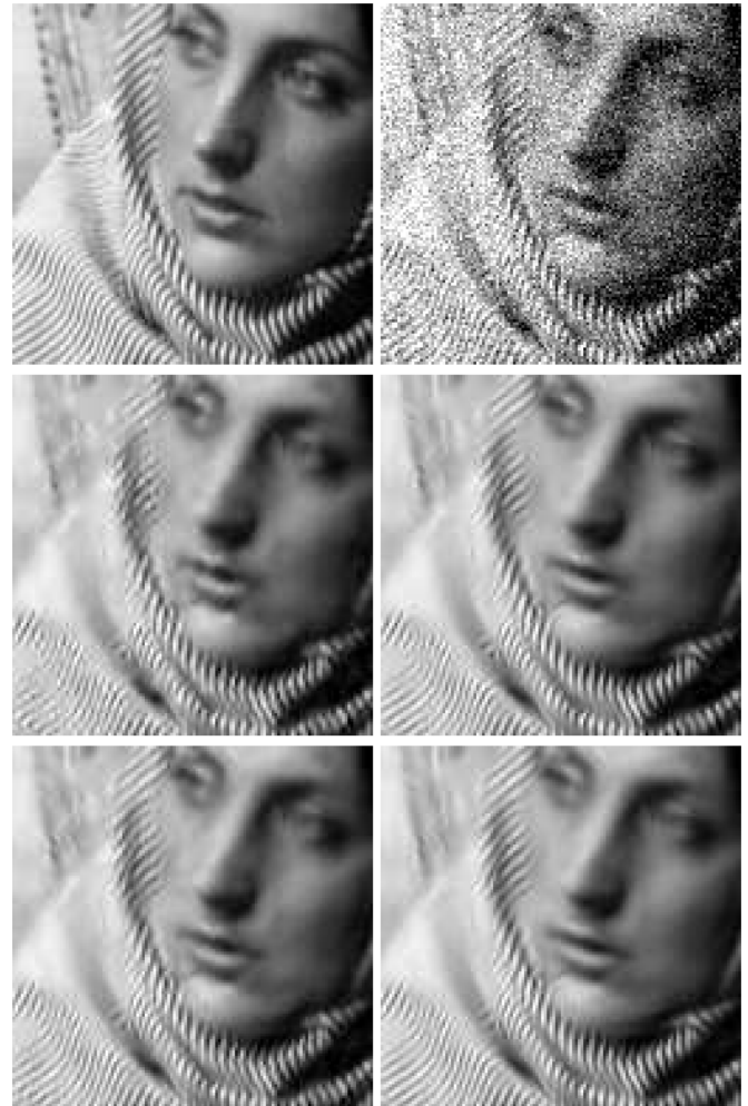
Fig. 5. 128 \times 128 detail from “Barbara” image, for noise with \sigma = 25 . Top: Original, noisy (20.17 dB). Middle: gsm2 (28.36 dB), oagsmnc2 (29.07 dB). Bottom: gsm8 (29.11 dB), oagsmnc8 (29.51 dB).
