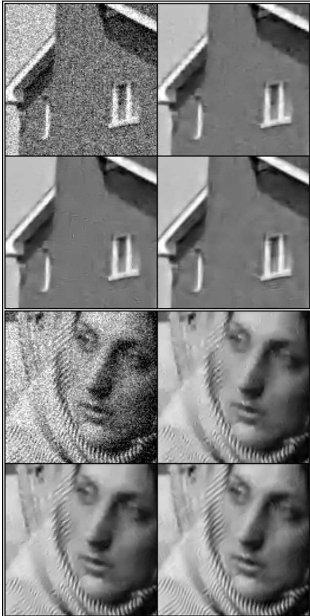
Fig. 2. Example denoised images. We compare three GSM-based methods, all implemented using TIHP, for House and Barbara images both with \sigma = 25 . Images are cropped to 128 \times 128 pixels for visibility (starting in pixel [24,64] and [288,64] respectively [column, row]). For each 2 \times 2 panel, from left to right and top to bottom the PSNR values ( House / Barbara ) are: noisy observation (20.17/20.17); BLS-GSM method [7] (31.59/27.81); SVGSM [8] (31.71/28.81); our MGSM result (32.12/29.80).
