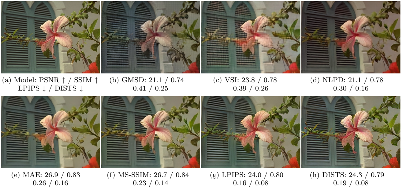
Fig. 14 A visual quality assessment example of compression. (a) Uncompressed image. (b)-(h) are the compressed results optimized for indicated IQA models. The results of MAE and MS-SSIM outperform the others in terms of PSNR and SSIM, but are not among the best judged by humans. LPIPS and DISTS are more consistent with human perception in this example.
