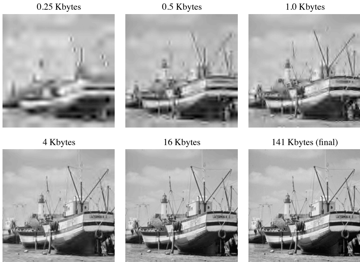
Figure 13: A progressive series of the Boats image, encoded using EPWIC-2. Data transmission amounts are given above each image.
