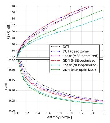
Fig. 3. Rate-distortion results averaged over the entire Kodak image set (24 images,  $752 \times 496$  pixels each). Reported rates are average discrete entropy estimates. Reported distortion is average PSNR (top) and distance in the normalized Laplacian pyramid domain (bottom – see text).
