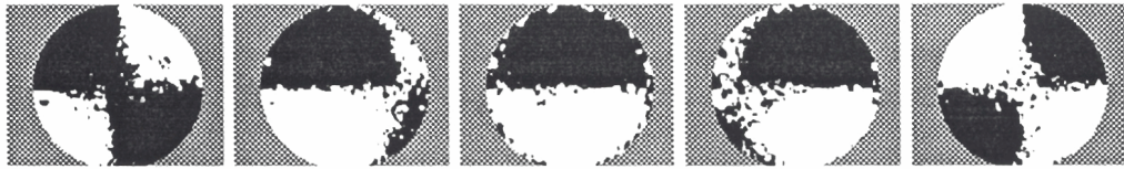
Figure 13: Real 180 Degree FOV Image Sequences. The sign of the longitudinal flow is depicted for different directions of heading; compare with the figure in the simulated experiment (Fig. 11). From left to right, the directions of heading are -90^\circ , -45^\circ , 0^\circ (direct ahead), 45^\circ and 90^\circ .
