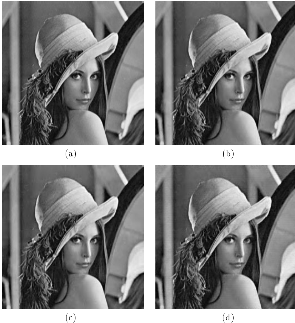
Figure 4.22: Data compression example using four-level pyramids. The pyramid data was compressed to a total of 65536 bits (i.e. total first-order entropy was 1.0 bit/pixel). (a) Original “Lena” image at 256 \times 256 pixels. (b) Compressed using 9-tap separable QMF bank. (c) Compressed using 3-tap asymmetrical filter bank. (d) Compressed using “4-ring” hexagonal QMF bank.
