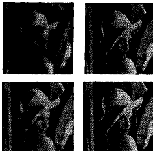
Fig. 15. Progressive transmission images using a four-level pyramid transform constructed with hexagonal filters. The first image is produced by reconstructing only the low-pass signal at the fourth pyramid level. The next image results from reconstructing the entire fourth level, or equivalently, the low-pass image on the third level. The final image is not shown.
