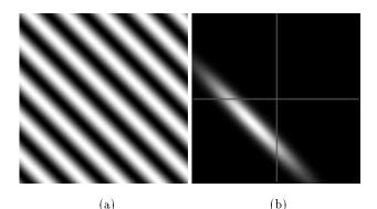
Figure 2: (a) One frame of a drifting sin grating sequence. The normal direction of the motion was down and to the left. The drift speed (in the normal direction) was 0.83 pixel/frame. (b) The response of the system computed over a patch near the center of the image. The peak of the response coincides with the actual normal velocity.
