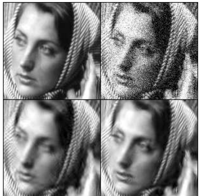
Fig. 6. Comparison of denoising results on Barbara image (cropped to 150 \times 150 for visibility of the artifacts). From left to right and top to bottom: Original image; Noisy image ( \sigma = 25 , PSNR = 20.2dB); Results of Li et al. [37] (PSNR = 28.2dB); Our method (PSNR = 29.1dB).
