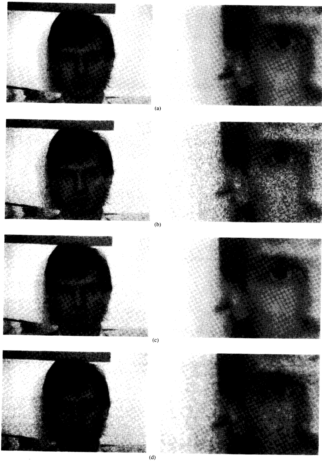
Fig. 15. Noise removal example. Figures on the right are enlarged portions of those on the left. (a) Original noise-free image. (b) Image corrupted by noise. SNR is 12.42 dB. (c) Results of image restoration using steerable pyramid. SNR is 23.0 dB. (d) Results of image restoration using a Wiener filter (see text). SNR is 19.24 dB.
