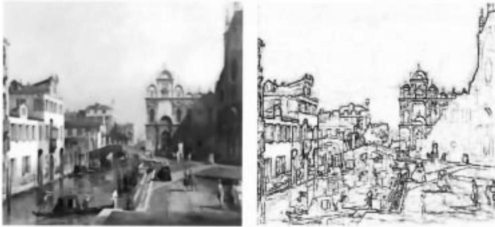
Fig. 14. Anisotropic diffusion with spatially coherent outliers. Left: smoothed image. Right: value of the line process at each point taken to be the product, l_{s,h}l_{s,v} , of the horizontal and vertical line process at s .
