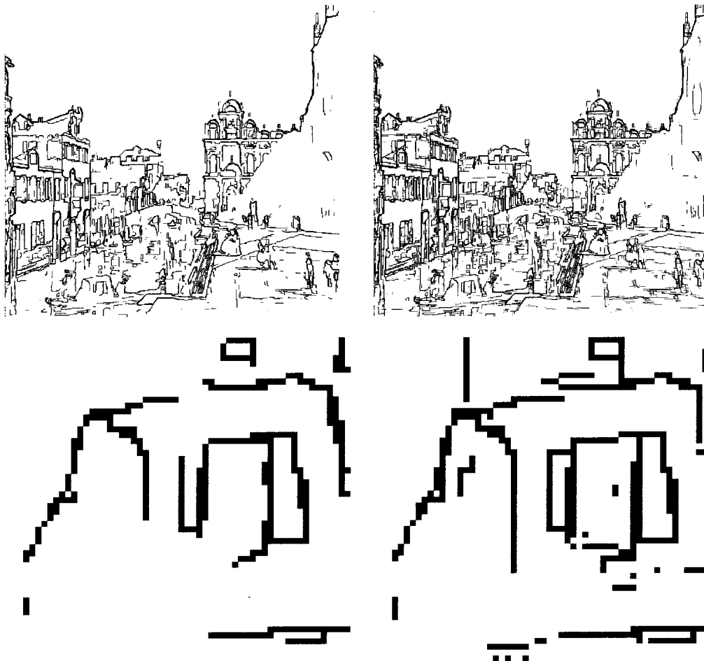
Fig. 15. Left: Edges obtained with Perona–Malik. Right: Perona–Malik with additional spatial coherence in the line processes. Lower images show details on the gondola.
